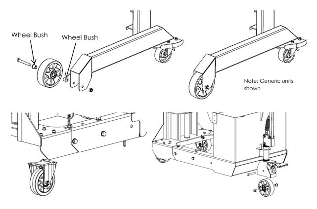
Use the same procedure as previously mentioned to replace the rear castors, ensuring that the wheel bushes are re-fitted in the wheel prior to re-bolting. For DTP08 models, the rear wheel used for steering will need to be jacked up high enough to allow it to be removed from the castor.
