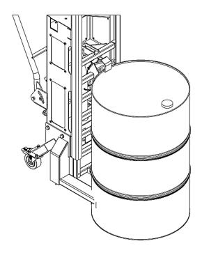
NOTE: THE DRUM LIFTER IS DESIGNED TO LIFT DRUMS OFF A EURO PALLET AND CANNOT LIFT DRUMS OFF THE FLOOR
