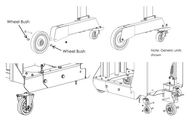
Use the same procedure as previously mentioned to replace the rear castors, ensuring that the wheel bushes are re-fitted in the wheel prior to re-bolting. For DTP08 models, the rear wheel used for steering will need to be jacked up high enough to allow it to be removed from the castor.
